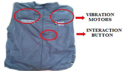
Fig. 13. Vibration motors and interaction button location.
