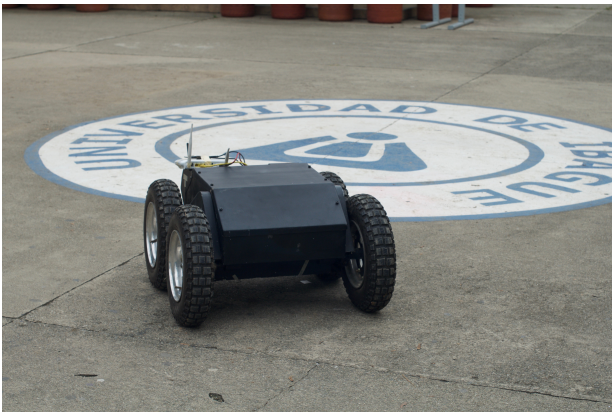
Fig. 4. The picture shows the Rover: A four wheel skid-steering mobile Robot.
